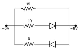
**Sol.** Below diode is in reverse bias so no current flow through it circuit looks like.
